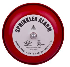
with minimum number of fittings. If the length of the pipe exceeds 22.8 mtrs. (75 feet), then higher size pipe must be used to reduce hydraulic friction loss. The Sprinkler Alarm should not be located more than 1.8 mtrs. (Six feet) above Alarm Valve / Deluge Valve.
