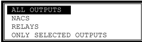
**Note:** “Strobes” can be added to the disable outputs pop-up window via the PC-Net field configuration programming tool, under “Disable Outputs Menu Options”.
