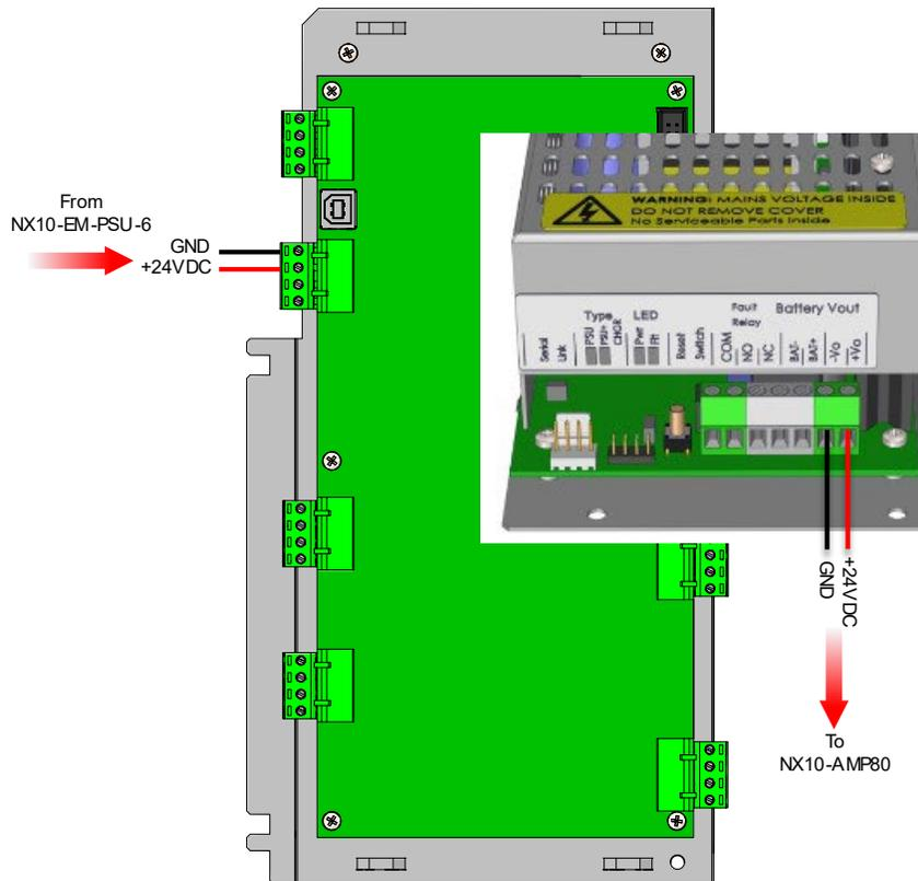
Figure 45 - NX10-AMP-80 24 VDC Wiring
