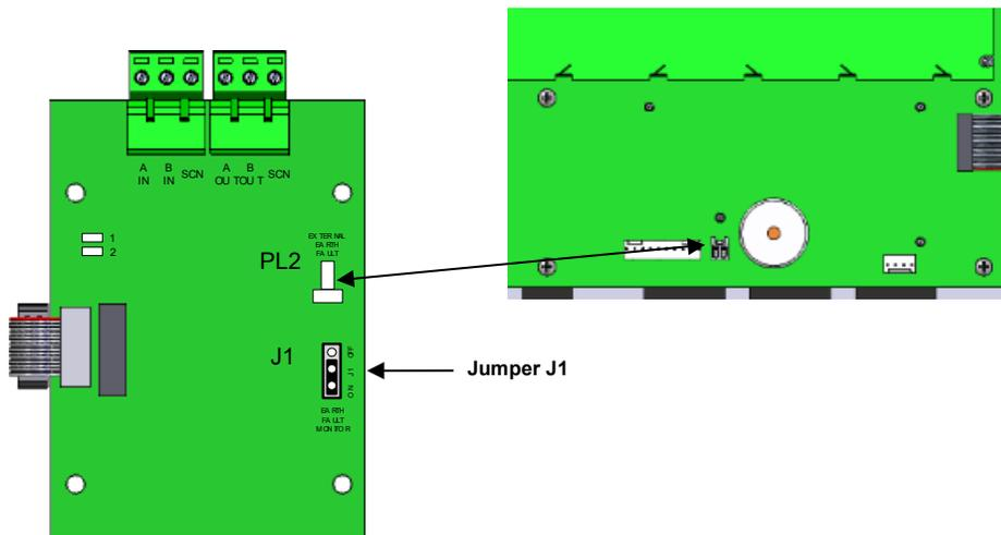
Figure 29 – NX10-FANET4 Network Ground Fault Detection Configuration
