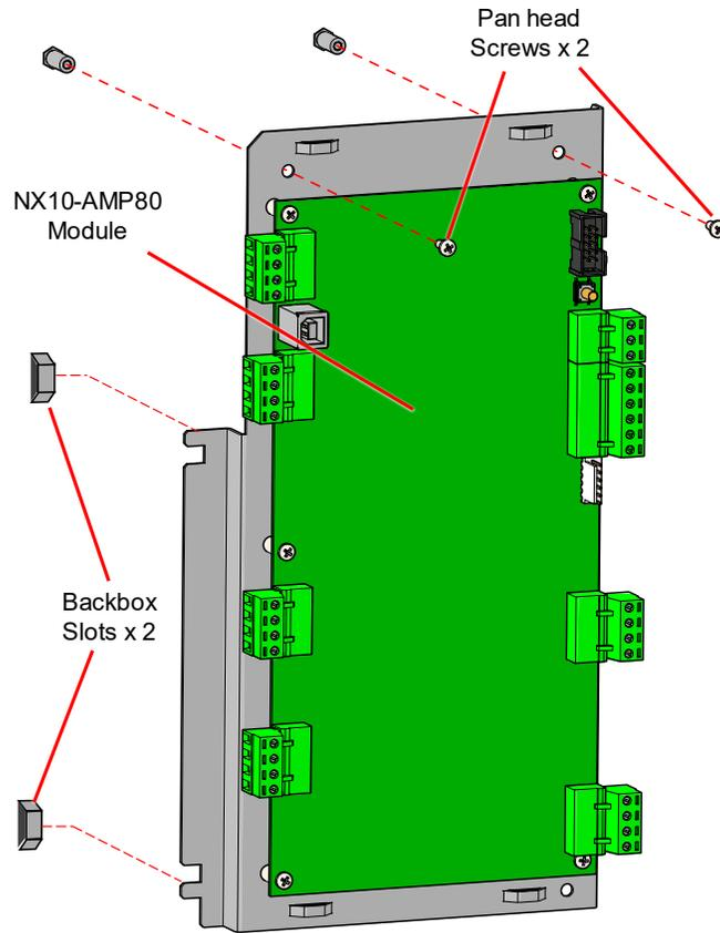
Figure 43 - NX10-AMP-80 Module Installation
