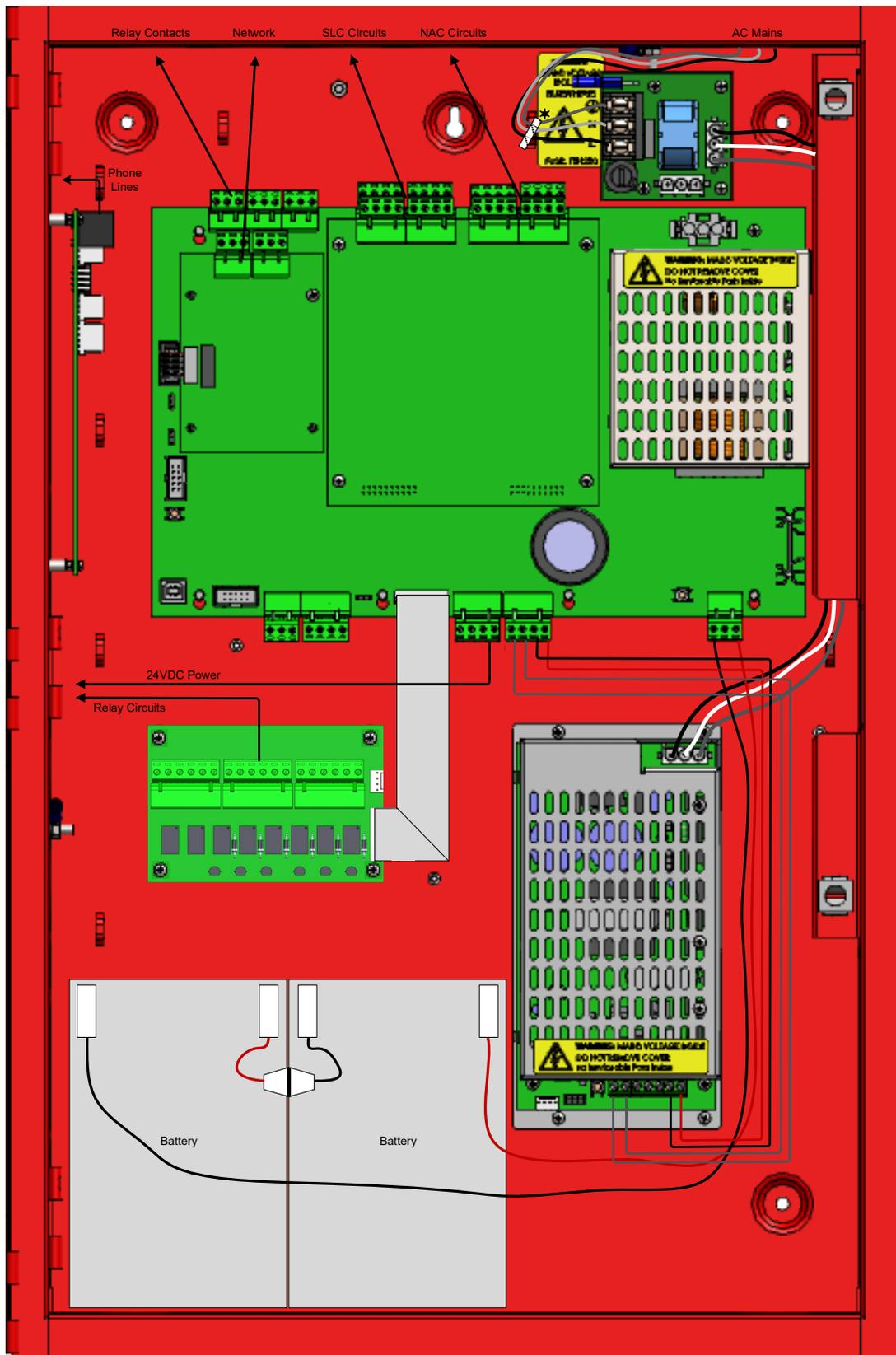
Figure 52 – NX10-FACP-(x) Wire Routing (NX10-FACP-4 shown)
