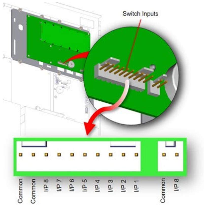
Figure 21 - NX10-ACS-DSP Switch Input Wiring
