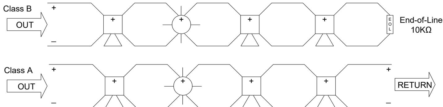
CAUTION: Break wiring run to maintain supervision of connections.
