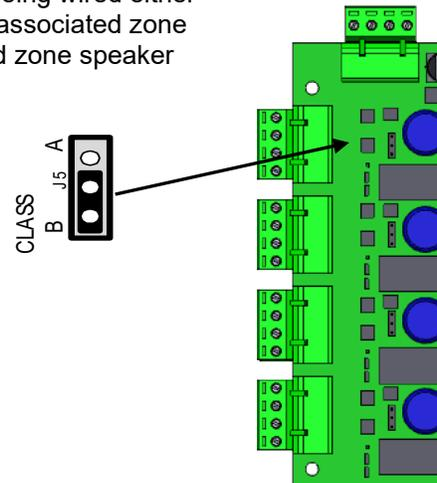
To wire speaker circuits of the zone splitter module, wire the B+ and B- terminals of the speaker circuit to the field installed speakers. If wired Class B, place the supplied 47K end-of-line (EOL) resistor at the last field speaker. If wired Class A, return the wiring of the last field speaker back to the A+ and A- terminals of the speaker circuit (Figure 37).
