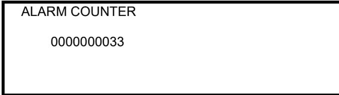
The FACP increments the alarm count each time it changes from the normal condition to an alarm state. While the panel is in alarm, if an additional alarm event occurs it does not advance the counter.
