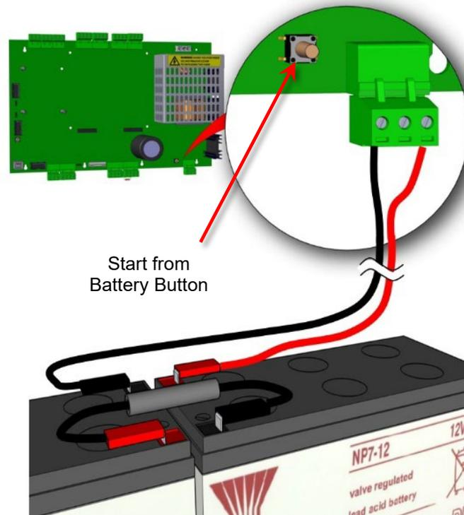
Figure 10 - Battery Connection
