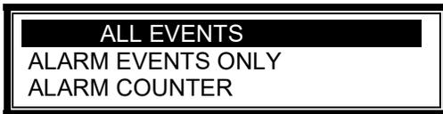
Press the  $\uparrow\downarrow$  buttons to highlight the required view option and then press the  $\checkmark$  button to select it. The display then shows the appropriate list of events.
