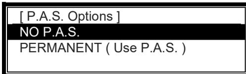
Highlight the required option using the ↑↓ buttons and then press the ✓ button to confirm. The display then reverts to the Main Menu.
