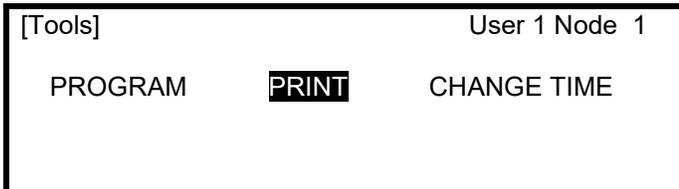
The data stream sent to a printer is in a serial format, if an external printer is used, make sure that the communications settings of the printer are set correctly.
