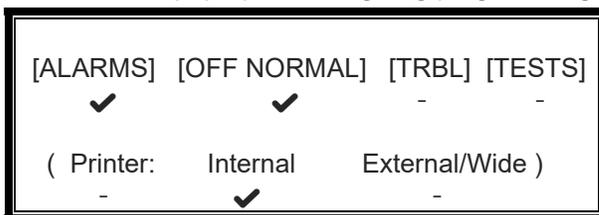
The upper line of options determines whether the panel will automatically print specific events as they occur. The lower line of options determines whether a printer is connected and the type of printer it is.
