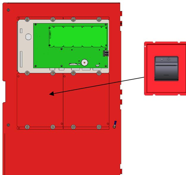
Figure 35 – NX10-EM-PRN Printer Module Installation
