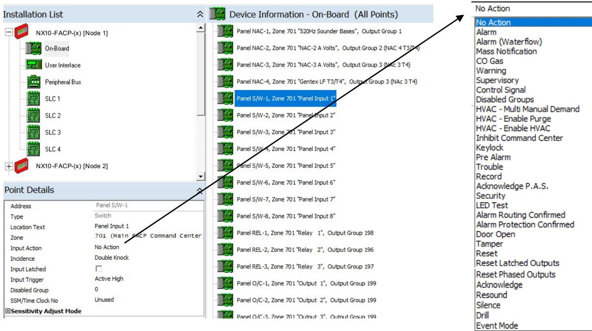
Figure 22 - Neo NX Config Tool, NX10-ACS-DSP Switch Input Programming
