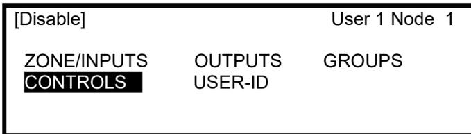
If the current User-ID (access level password) does not have the required authority, the display prompts for entry of an authorized password to guard against inadvertent changes.
