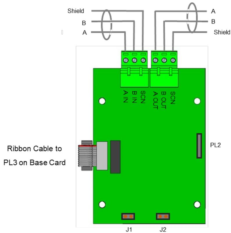
Figure 28 - NX10-FANET4 and NX10-FANET7 Wiring
