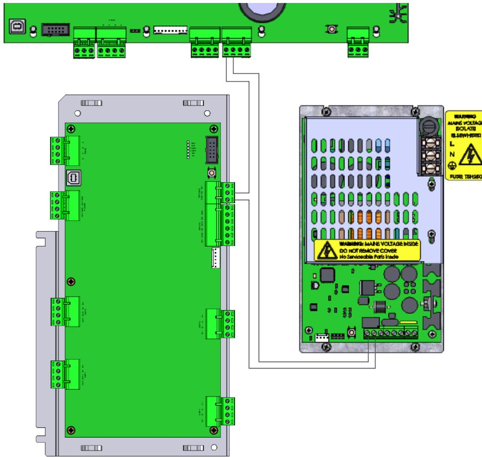
Figure 49 - Hardwired Audio Amplifier and Power Supply Charger Supervision Wiring
