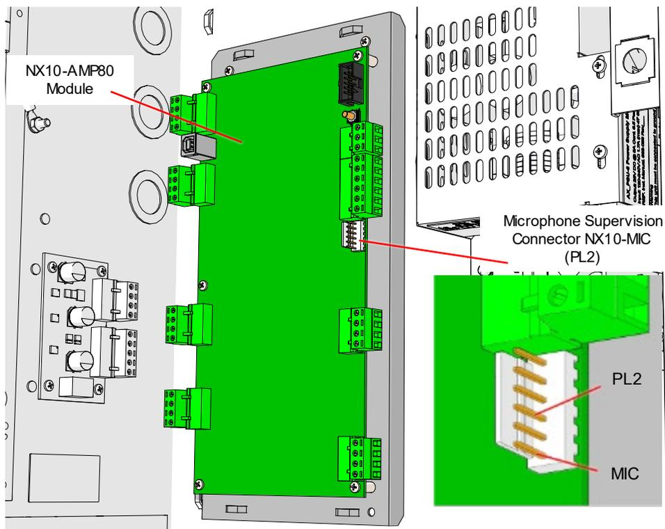
Figure 44 - Connector NX10-MIC-PL2
