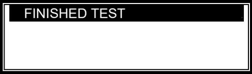
Selecting the FINISHED TEST option will cancel all zones that are in test mode. The Test LED will then extinguish. If there are any zones still in a test or alarm condition, a pop-up window with the following options will appear:
