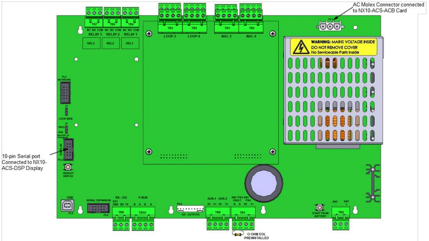
Figure 8 – NX10-FACP-2 Two-Loop Base Card with NX10-EM-LPD SLC/NAC Expansion Module (NX10-FACP-4)
