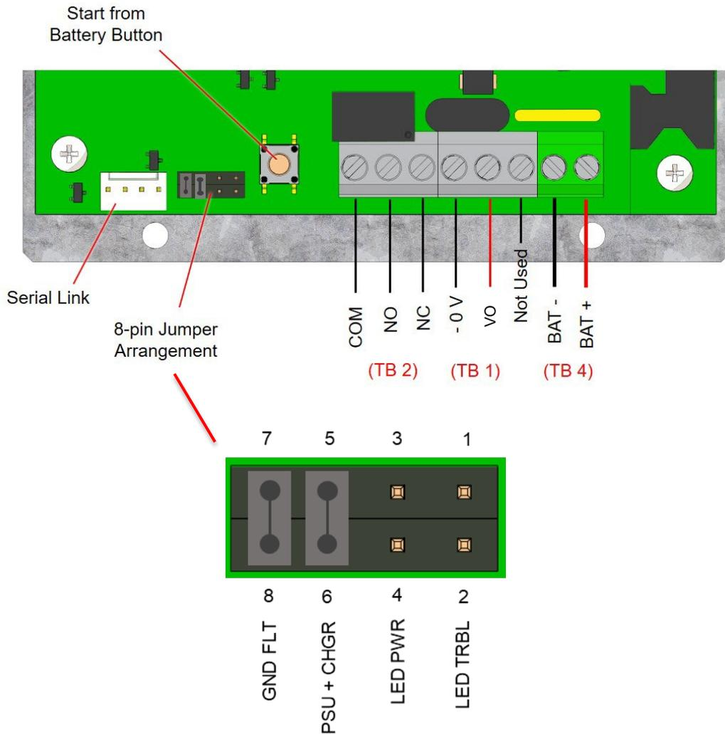
Figure 31 - NX10-EM-PSU6 Connections
