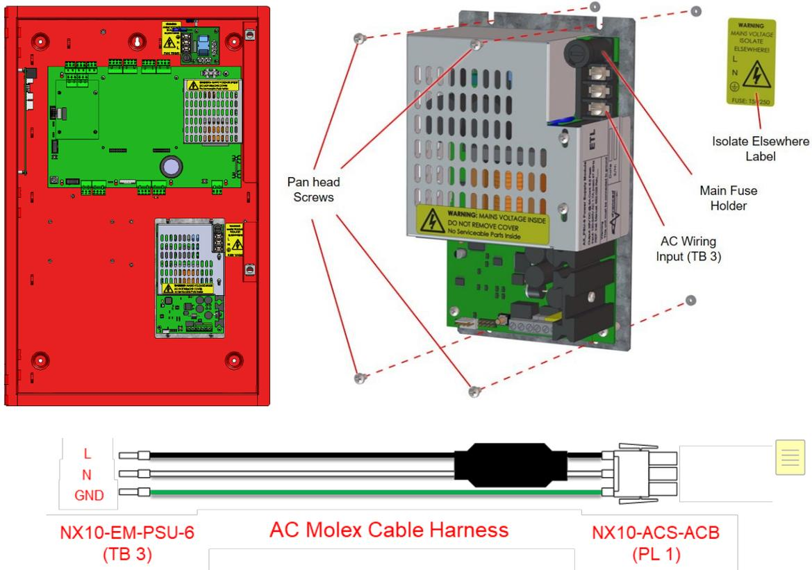
Figure 30 – NX10-EM-PSU6 Module Installation
