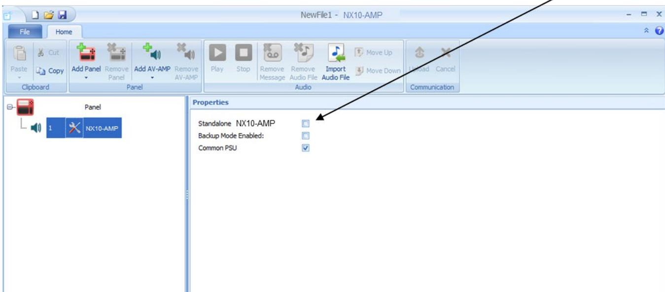
Figure 51 - Audio Amplifier Backup Programming
