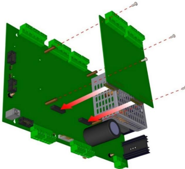
Figure 14 - NX10-EM-LPD Module Installation to an NX10-ACS-2L Base Card
