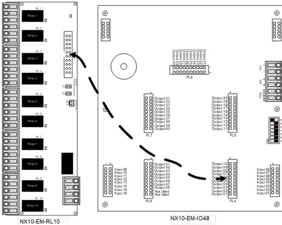
Figure 23 - NX10-EM-RL10 to IO48 Interface
