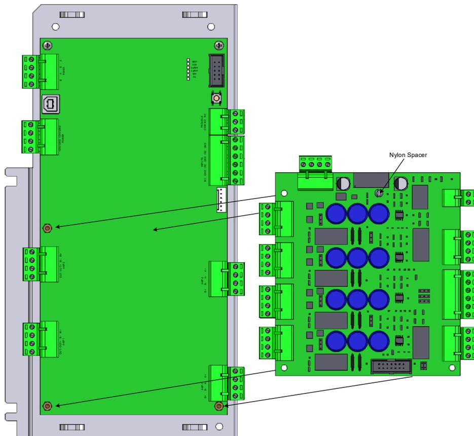
Figure 33 – NX10-ZS Module Installation
