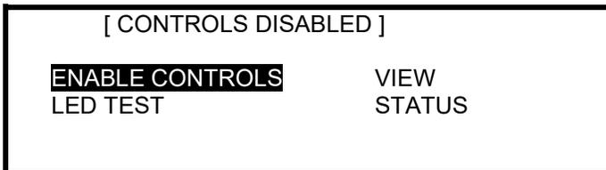
The display will automatically revert to the normal operating display after 15 seconds.
