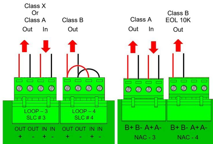
Figure 15 - NX10-EM-LPD SLC and NAC Wiring
