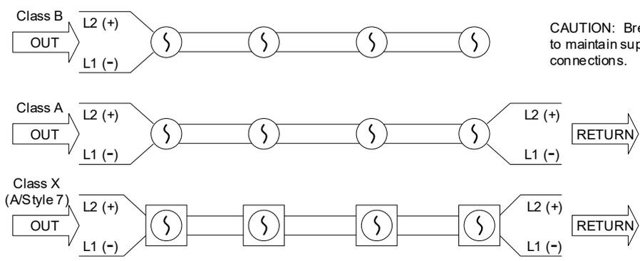
CAUTION: Break wiring run to maintain supervision of connections.
