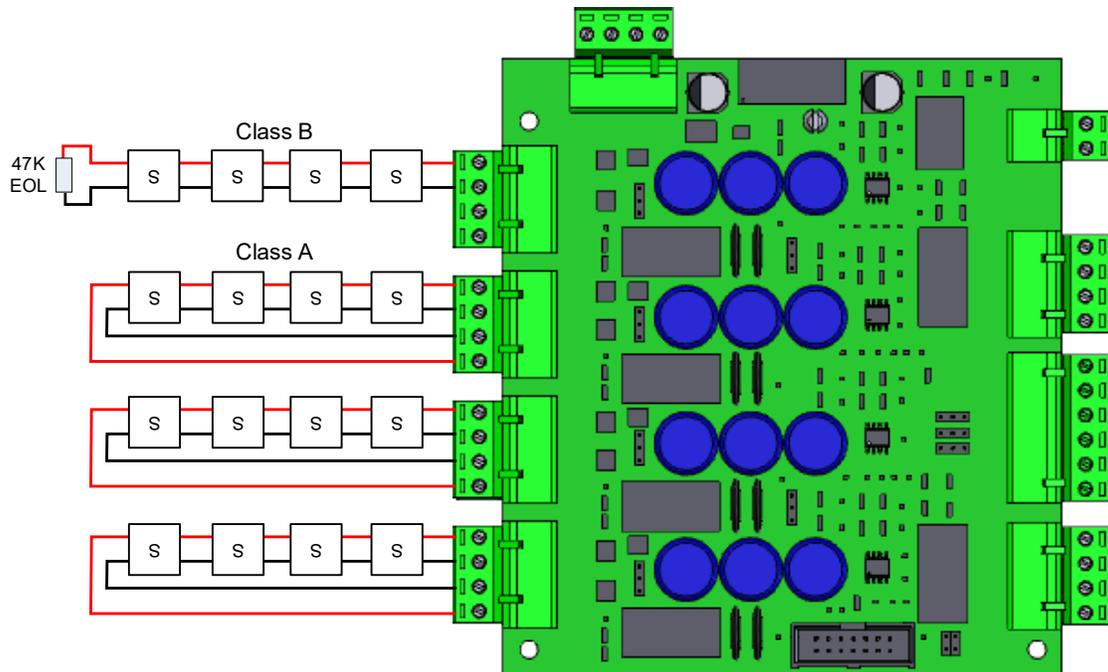
Figure 34 -NX10-ZS Speaker Circuit Wiring
