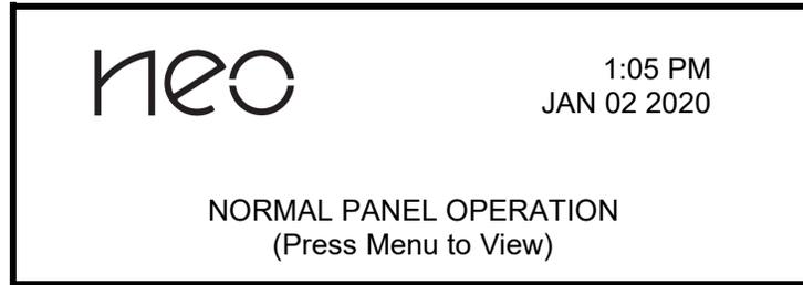
The graphical LCD display provides detailed information on the operational status of the FACP. Above is an example of the normal standby state of the display.
