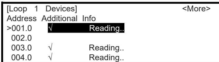
When the reading is complete, the display will show the drift (0-100%) per intelligent smoke detector on the SLC loop.
