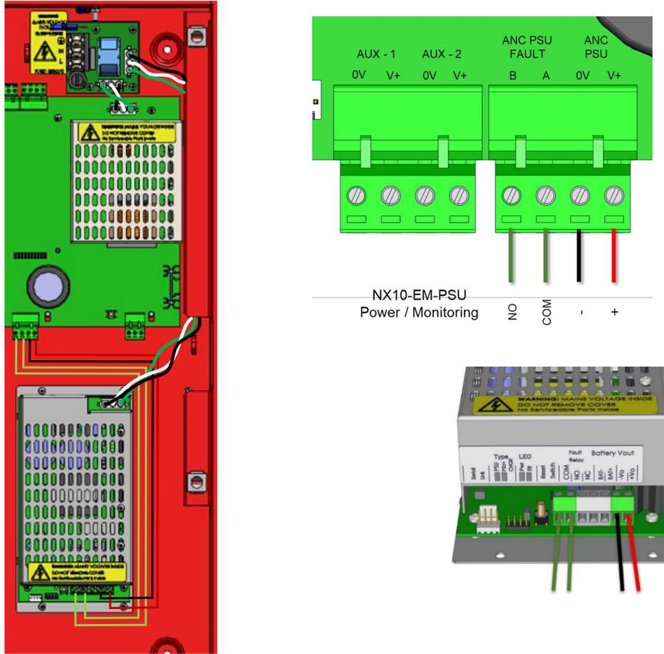
Figure 17 – NX10-EM-PSU Module Installation and Wiring
