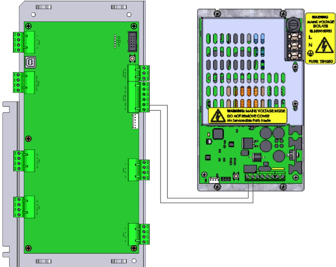
Figure 48 - Peripheral Bus Audio Amplifier NX10-EM-PSU6 Monitoring
