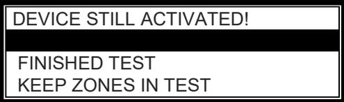
Alternatively, it is possible to leave the Test – Zone’s sub menu with one or more zones still in test mode by selecting the KEEP ZONES IN TEST option. This will enable the use of other menu functions and return the display to the normal operating mode. The Test LED will stay illuminated if this option is selected.
