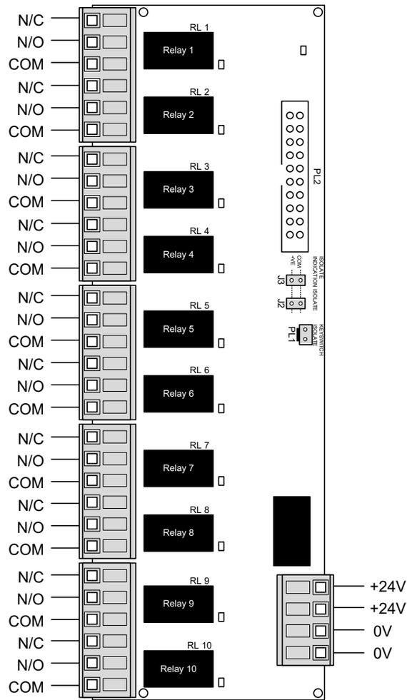
Figure 26 - NX10-EM-RL10 Wiring
