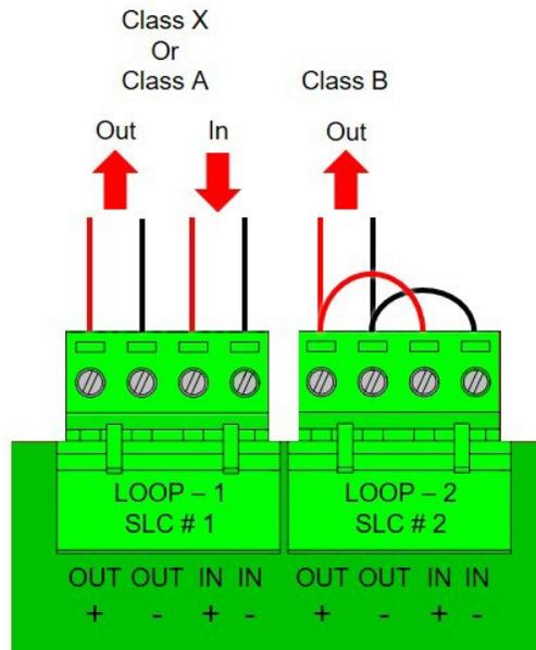
Figure 12 - Base Card SLC Circuit Wiring
