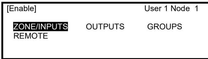
Press the ←→, ↑↓ buttons to highlight the required sub menu option and then press the ✓ button to select it.
