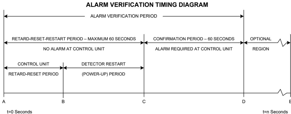
Alarm Verification provides a mechanism to delay an alarm from a smoke detector due to transitory events. It should not, however, be used as a substitute for proper detector location/application or regular system maintenance.
