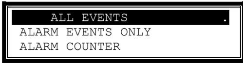
Press the  $\uparrow\downarrow$  buttons to highlight the required menu option and then press the  $\checkmark$  button to select it. The display then shows the appropriate list of events.
