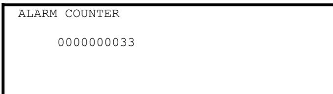
In the above example, the panel has entered an alarm condition 33 times since it was installed or since last log erase.
