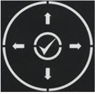
UP, DOWN, LEFT and RIGHT arrow keys are used to scroll through multiple status events, device details, and to navigate through the various displays and menus.
