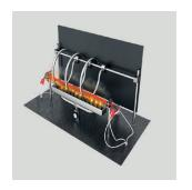
The cable is exposed to fire at the  $950^{\circ}$ C for 180 minutes.
