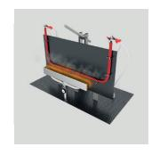
This test is carried out to verify the circuit integrity of cables exposed to fire at 830°C and mechanical shocks.
