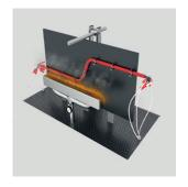
The cable is mounted on a vertical panel and shocked with a steel bar for 15 minutes while submitted to the action of a flame
