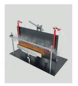
This test is carried out to verify circuit integrity during a fire. The cable is exposed to a flame at 930°C and mechanical shocks for 60 minutes and additional 60 minutes to flame, mechanical shocks and water spray.
