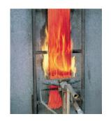
Samples of cables 3,5 m long in quantities required by standard are installed on a ladder inside a metallic cabinet. They are subjected to the action of a flame at 750°C for a specific time (20 or 40 minutes). Cables must not burn for more than 2.5 m
