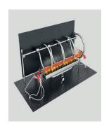
This test is carried out to verify circuit integrity even during a fire. A sample of cable is held on a flame at about 750°C for a period of minimum 90 min, under rated voltage.
