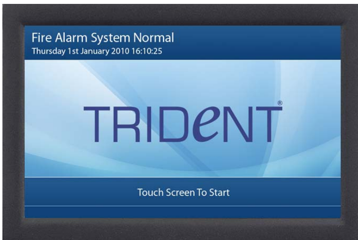
Figure 1-2 Normal-Standby-Condition of Touch-Panel-Display
