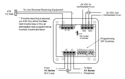
Figure 36 - Reverse Polarity Wiring
