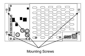
Figure 28 - NX-EM-PSU6 Power Supply Charger Module
