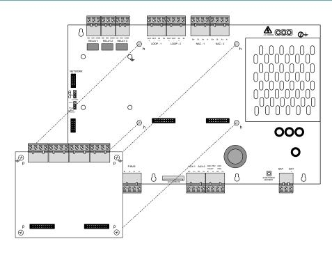
Figure 29 - NX-EM-LPD or NX-NAC Module Mounting to NX-ACS-2L
