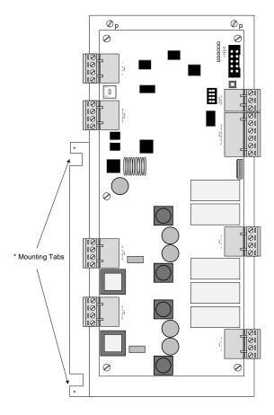
Figure 24 - NX-AMP-80 Audio Amplifier Module Mounting
