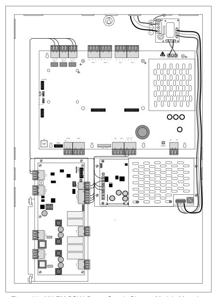
Figure 27 –NX-EM-PSU6 Power Supply Charger Module Mounting
