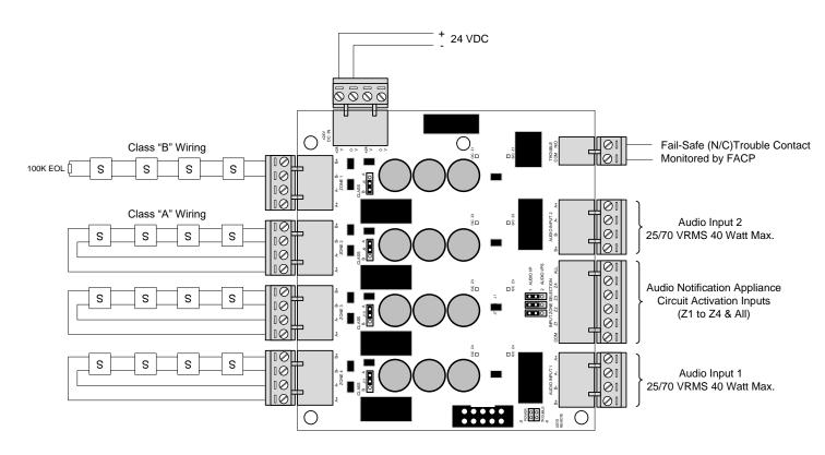
Figure 26 -NX-ZS Audio Zone Splitter Module
