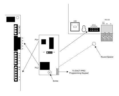
Figure 32 - NX-SEB to D9068P Wiring
