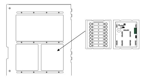
Figure 37 - Switch/LED Module Installation
