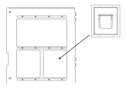
Figure 45 - NX-EM-012 Panel Printer
