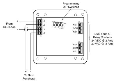
Figure 16 - S-A4050 Wiring
