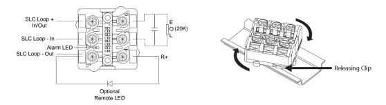
Figure 8 - S-A4041 Wiring & Optional Mounting
