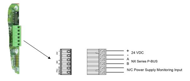
Figure 39 - Switch LED Module Wiring
