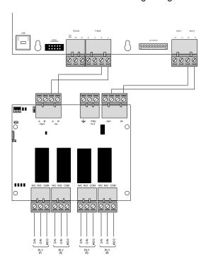
Figure 41 - NX-EM-RL4 NEO Enclosure Mounting
