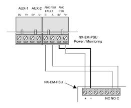
Failure to tighten the screws will defeat the protection circuitry designed to protect the module from damage due to lightning and static electricity.
