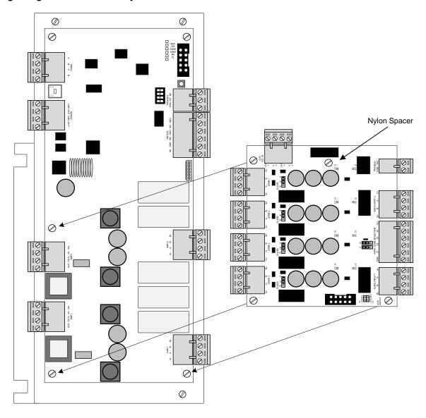
Figure 25 - NX-ZS to NX-AMP-80 Mounting
