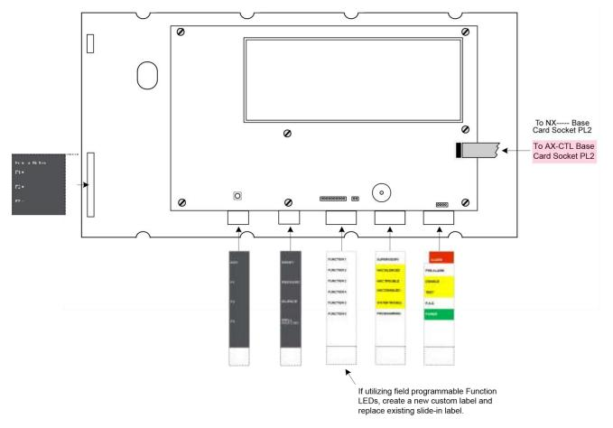
Figure 19 - Slide-in NX-ACS-DSP Labels
