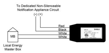
If replacing an NX-CTY module, simply disconnect the field wiring from the NX-CTY wire leads and reconnect the field wiring to the new NX-CTY module wire leads.
