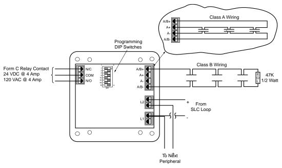
Figure 13 - S-A4049 Wiring
