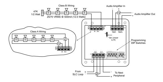
Figure 15 – S-A4046 Speaker Circuit Wiring
