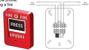
The S-A4061, Intelligent Dual Action Polycarbonate Pull Station, can be mounted semi-flush onto a standard single-gang electrical outlet box. If installations require surface mounting, an optional polycarbonate surface back box (S-A4062) is available.
