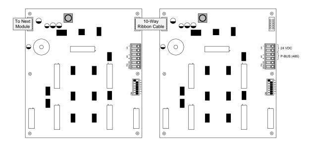
Figure 40 - Switch LED Module Daisy Chain Wiring
