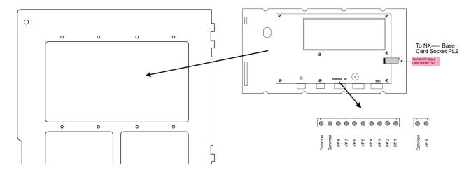
Figure 20 - NX-ACS-DSP Installation and Inputs
