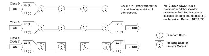
Note: During normal operation the panel will drive the SLC from the OUT connections, if a short circuit or open circuit condition is detected it will drive the SLC from both OUT and IN (RETURN) sides. During programming mode, the panel will drive the SLC from the OUT connections only to enable easier wiring trouble diagnosis.
