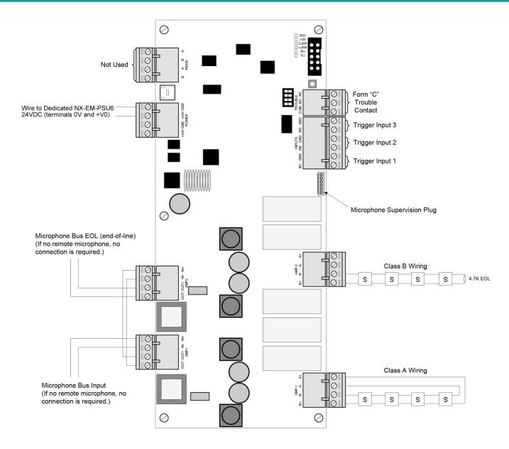
Figure 22 - Hardwired NX-AMP-80 Amplifier
