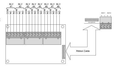
The NX-EM-RL4 four point relay output module is an optional PBUS (RS485) module for use the NX-FACP-1L, NX-FACP-2 or NX-FACP-4 intelligent fire alarm control panel's NX-FACP base card. The NX-EM-RL4 provides four (4) fully field programmable Form "C" relay contacts for project specific control functions. The NX-EM-RL4 is listed to switch DC or AC voltage and up to sixteen (16) NX-EM-RL4 modules can be connected to a single NX-CTL base card providing a maximum of 64 relay outputs.
