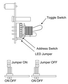
Available in either single (NX-APS2-F1) or dual (NX-APS2-F2) action configuration, the NX-APS2-xx stations are designed to prevent false alarms when bumped, jarred or shaken. The dual action NX-APS2-F2 further deters malicious false alarms by requiring a two-process function for activation; first push the "PUSH" bar inwards which then allows the "PULL" bar to be grasped and pulled outward.
