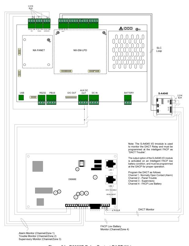
Figure 34 - D9068E Relay Contact DACT Wiring
