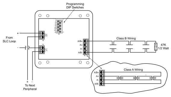
Figure 10 - S-A4043 and S-A4044 Wiring
