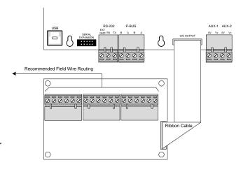
Failure to tighten the screws will defeat the protection circuitry designed to protect the module from damage due to lightning and static electricity.
