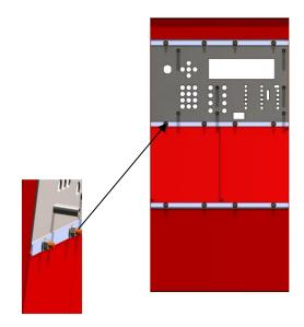
Figure 3- Aperture Installation
