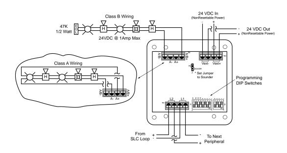
Figure 14 - S-A4046 Notification Appliance Circuit Wiring
