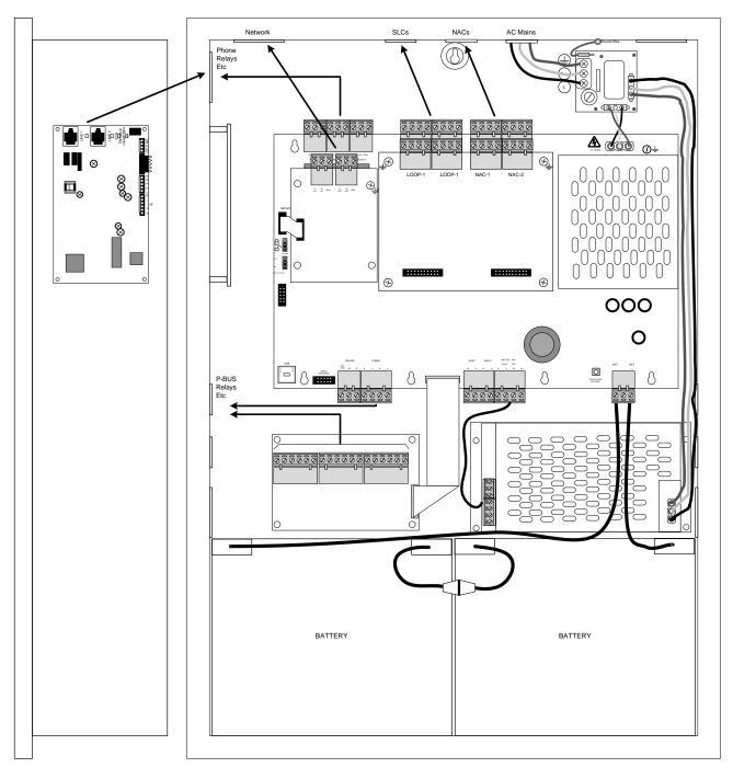
Figure 46 - NX-FACP-1L, NX-FACP-2 or NX-FACP-4 Cable Routing
