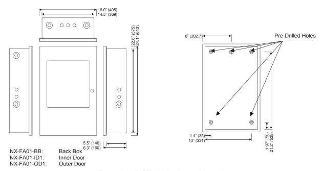
Figure 1 - NX-CTL-(x) Enclosure Dimensions
