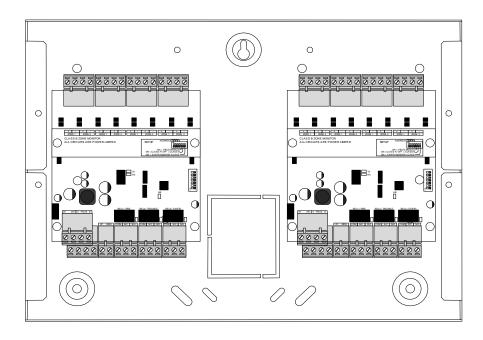
Figure 44 – NX-CZM NX-FA-009 Enclosure Mounting
