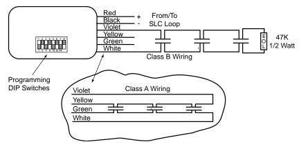
Figure 9 - S-A4048 and S-A4047 Wiring
