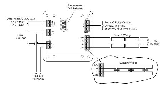
Figure 12 - S-A4045 Wiring
