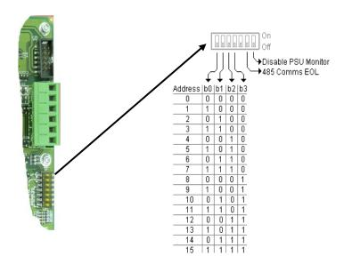
Figure 38 – Switch LED Module Addressing
