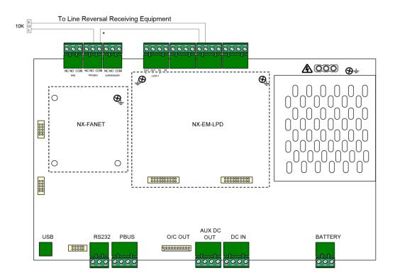
\* If trouble reporting is required, run A/B+ thru either the Base Card trouble relay or thru an addressable relay programmed as inverted, trouble activation.
